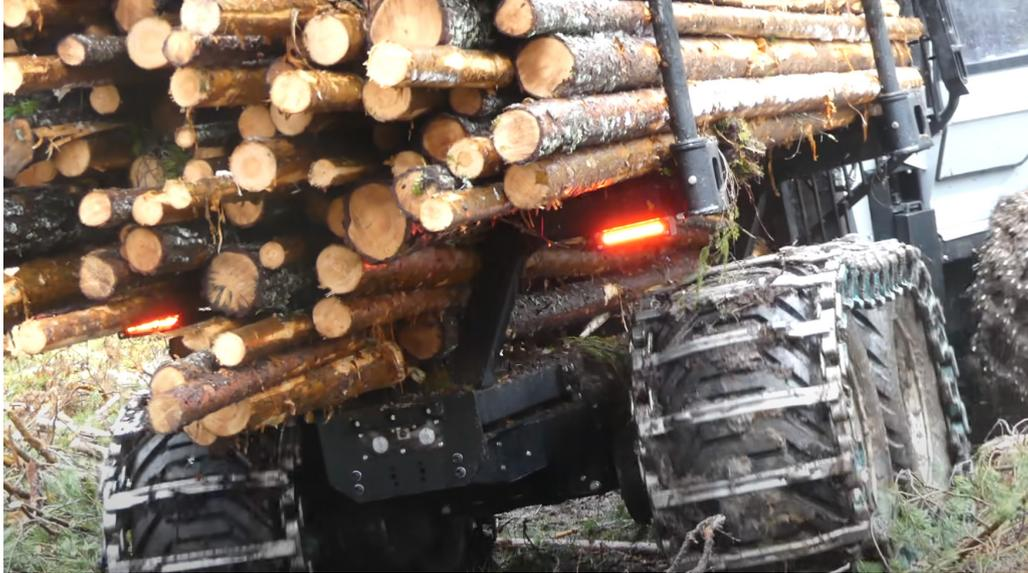
Vimek 870.1 NG has DSS (Dual Steering System), this means steering in both middle joint and rear boggie. This reduce the space required to operate Vimek 870.1 NG in stands.
